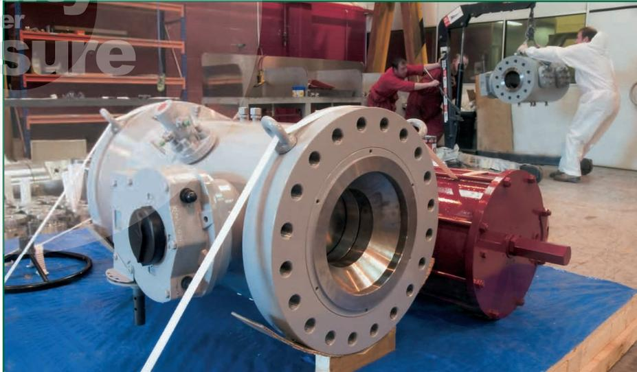
A Single Isolate 6" Full Bore 1500 LB Ball Valve to ASME B16.10 Length Versus An Oliver Twinsafe 6" Full Bore 1500 LB Double Block and Bleed Valve to ASME B16.10 Length.
